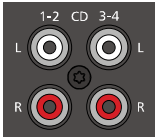
Illustration 2-12: RCA inputs CD 1-2 and 3-4
