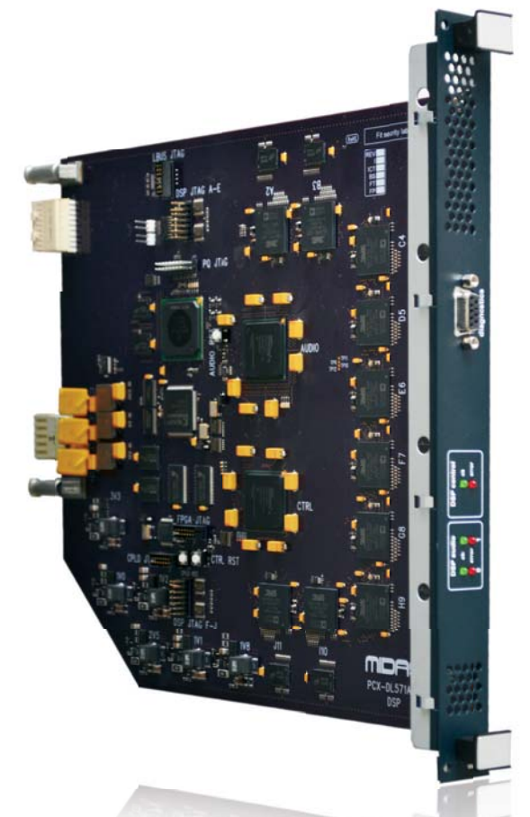
The nucleus of the NEUTRON is a Super Audio Engine that can process up to 800 audio paths.
