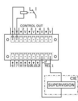
Figure 6.4: Connecting a relay and the supervision contacts of a CIE to the CONTROL OUT port
