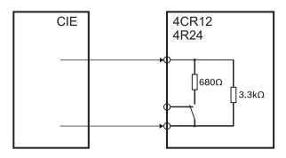
Figure 6.5: Internal configuration of the REL contact (VDE 0833-4)
