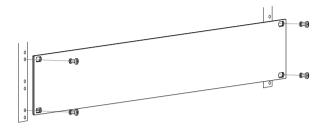
Figure 5.1: Installation of the device into a 19" rack
