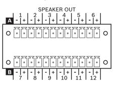
The audio outputs on the device allow to connect 100 V (or 70 V) loudspeaker zones. The delivery includes 12-pin connectors. Conductor cross-sections of 0.14 mm<sup>2</sup> (AWG26) to 1.5 mm<sup>2</sup> (AWG16) can be used.
