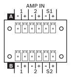
The AMP IN audio inputs allow to connect the 100 V (or 70 V) output signals of up to eight power amplifier channels to the integrated 2-in-6 router blocks A, B, C or D. Additionally there are four input channels for spare amplifiers.
