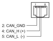
Figure 6.1: Assignment of the CAN port
