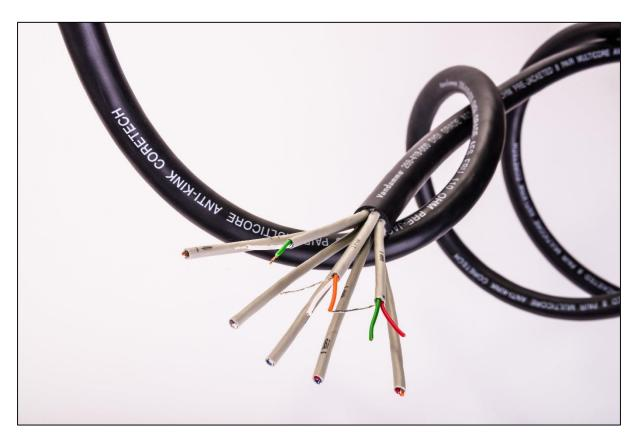
The Van Damme Digitour cables are black jacketed versions of the Green Series AES Microphone cable and 2, 4, 8 and 12 pair pre-jacketed multicores, introduced in response to user requests. Green Series is often used for DMX512 control signals, but lacks the unobtrusive jacket colour often needed by the Lighting and Presentation markets. Low capacitance and stable characteristic impedance make these cables ideal for DMX512 as well as AES/EBU and analogue audio signals
