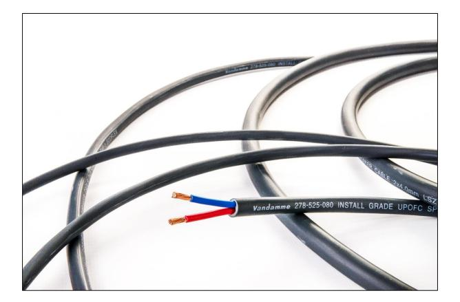
Van Damme Ecoflex Install Grade Twin Axial Speaker Cable LSZH is a Low Smoke Zero Halogen insulated and jacketed cable range. it is specifically designed for installation in public buildings and other areas where LSZH materials are specified such as new-build housing and marine installations. From 2 x 0.75 mm<sup>2</sup> for 100V line to 2 x 4.00 mm<sup>2</sup> for low impedance systems most speaker applications are well catered for.
