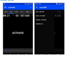
The Android version keeps all settings on the same page and allows the user to toggle between the activation buttons for each setting. The activation button must be long pressed to activate. The Android version also allows users to keep a configurable list of full sets of settings.
