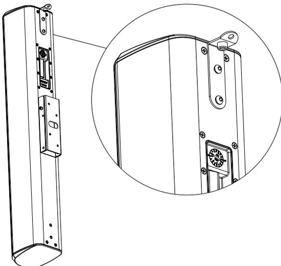
**Pan-Tilt Bracket (optional)** – A pan-tilt bracket is available which allows panning and tilting for flexible orientation along both horizontal and vertical axes. Detailed installation instructions are included with the pan-tilt bracket.
