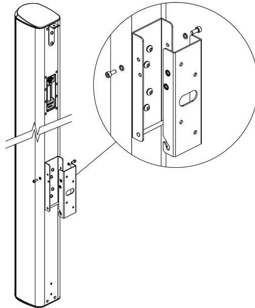
**Flying Bracket** – Each VLS Series loudspeaker is also supplied with a flying bracket. The bracket is attached to the top two inserts using the supplied M6 screws (Fig.5). The two bottom inserts can be used as pull back if required.
