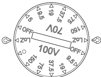
A multi-position rotary switch on the rear input panel selects either the low-impedance operating mode or the high-impedance modes (70 V or 100 V) with available transformer taps. When using VLS Series loudspeakers in distributed line systems, the transformer can be tapped with available power levels shown in the table below:
