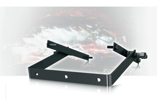
The NuQ82-FY is a matt black, powder coated flying yoke specifically designed to hang the NuQ82 in standalone applications, such as ceiling mounting in bars or clubs, or as an under-balcony fill. The NuQ82-FY consists of: a fly yoke; a pair of side plates, which attach to the sides of the loudspeaker; and a pair of plastic handle screws that secure the fly yoke to the side
